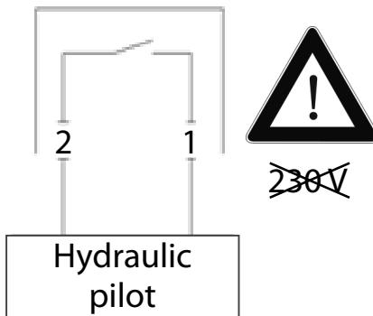
The input of the electronic card for the connection of the room thermostat is potential free (dry contact). Do not connect a power supply.
