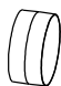
1 connecting sleeve for extension pipe to connect to insulated extension pipe or insulated elbow
