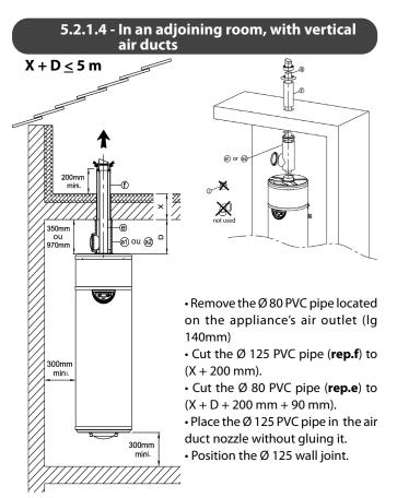
• If the Ø 80 PVC pipe is short enough to pass through the top, insert it into the Ø 125 PVC pipe. Pass the nozzle, assembled with the Ø80 PVC pipe (the Ø 125 PVC pipe must not overlap on the inside) through the adjoining room. Make sure that the Ø 80 PVC pipe passes through the wall flange and the insulated elbow, (see below, depending on dimension «D» you may need to extend it).
