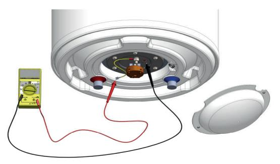
If the current is >0.3mA, the anode is operational, if the current <0.3mA check the anode visually.
