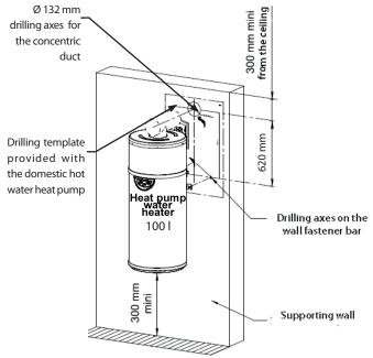
\* In the case of assembly with horizontal air ducts or with Ø 80 mm PVC pipe (with direct outlet at the back)
