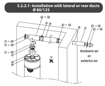
Close-up for assembly of the insulated elbow
