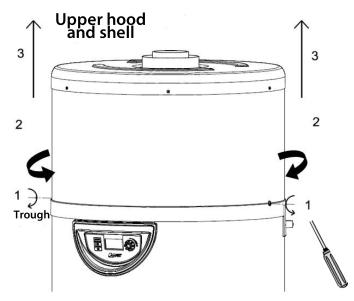
To access the heat pump and the electrical connections you will first need to partially dismantle the air duct, starting with the Ø80 inside pipe and then the insulated elbow:
