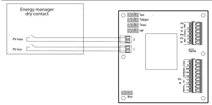
This function enables the appliance to operate in auto-production mode, which means that it will use the energy produced by the PV function to supply the heat pump as well as the electrical back-up, and to heat the water in the tank.
