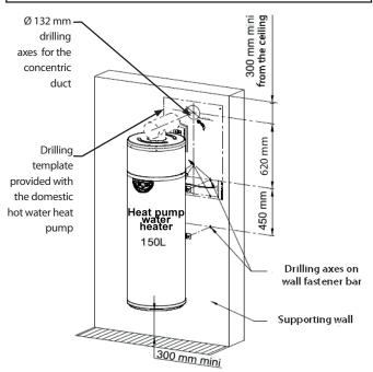
Reposition the domestic hot water heat pump and adjust the wall bracket(s) so that they are vertical. It is acceptable for the appliance to lean slightly to the right (max. 20 mm) or backwards (max. 10 mm), as the condensates outflow is located on the right-hand side at the rear of the appliance.
