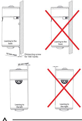
The vertical positioning of the domestic hot water heat pump must be strictly respected. If it is not, condensates could overflow and water may leak out onto the floor.
