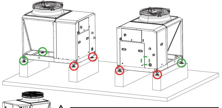
The two reinforcements (see illustration below, dotted red) are placed with the hydraulic adapters in the kit inside the heat pump. (See diagram below). They must be fitted (on the compressor side) before the springs are installed on the heat pump.
