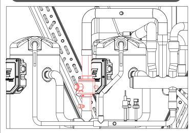
The HRC $^{70}$  40 kW tri V only has a shut-off valve for manufacturing the product on the assembly line. **This valve must never be closed.** Any damage to the machine caused by tampering with this valve will invalidate the machine warranty.
