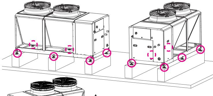
The two reinforcements (see illustration below, dotted red) are placed with the hydraulic adapters in the kit inside the heat pump. (See diagram below). They must be fitted (on the compressor side) before the springs are installed on the heat pump.
