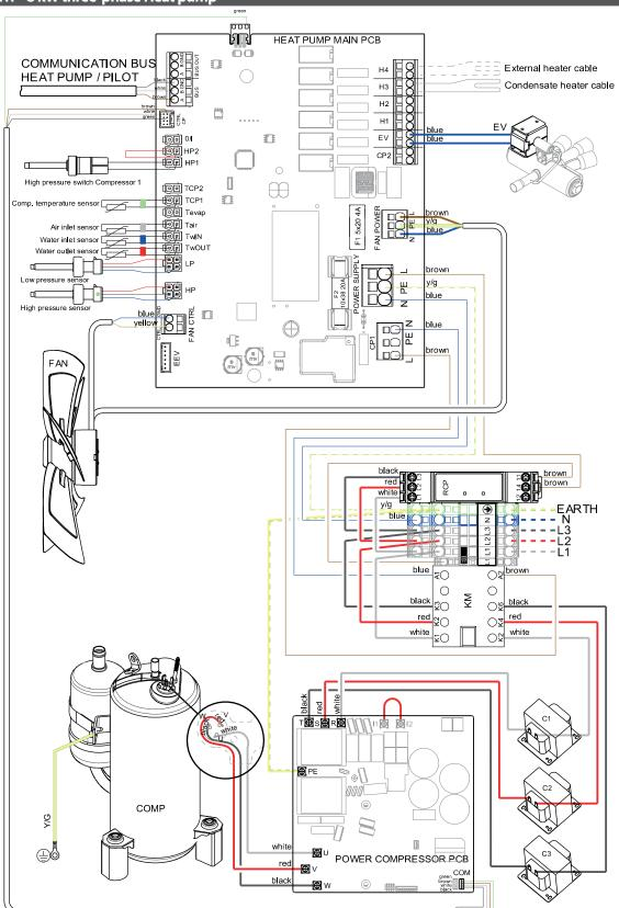
TwOUT- Water outlet temperature sensor
