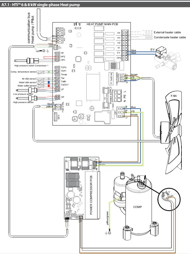
TwOUT- Water outlet temperature sensor
