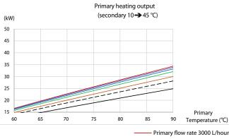
Primary flow rate 2500 L/hour Primary flow rate 2000 L/hour Primary flow rate 1500 L/hour Primary flow rate 1000 L/hour — - Primary flow rate 750 L/hour - Primary flow rate 500 L/hour
