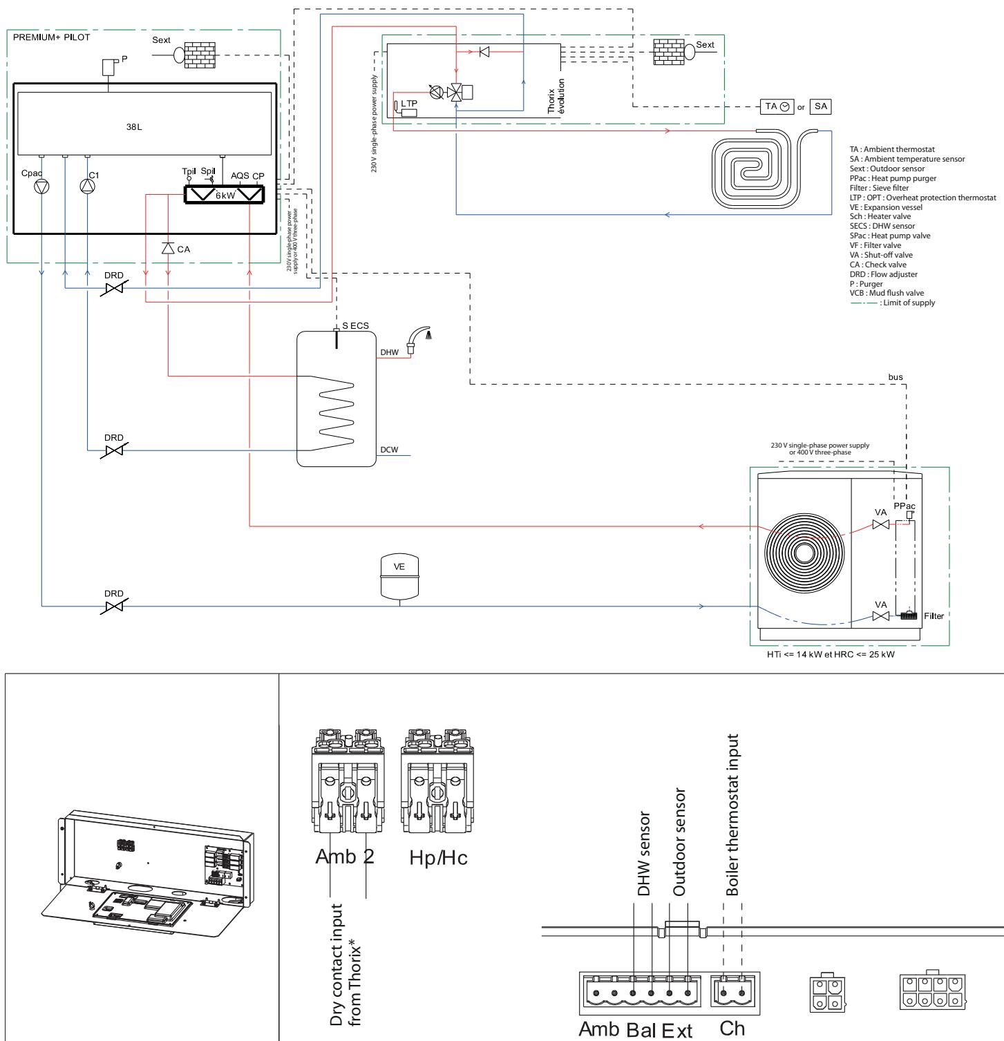
When there is a simultaneous demand on the heating and DHW circuits, both circuits are distributed at the same time.
