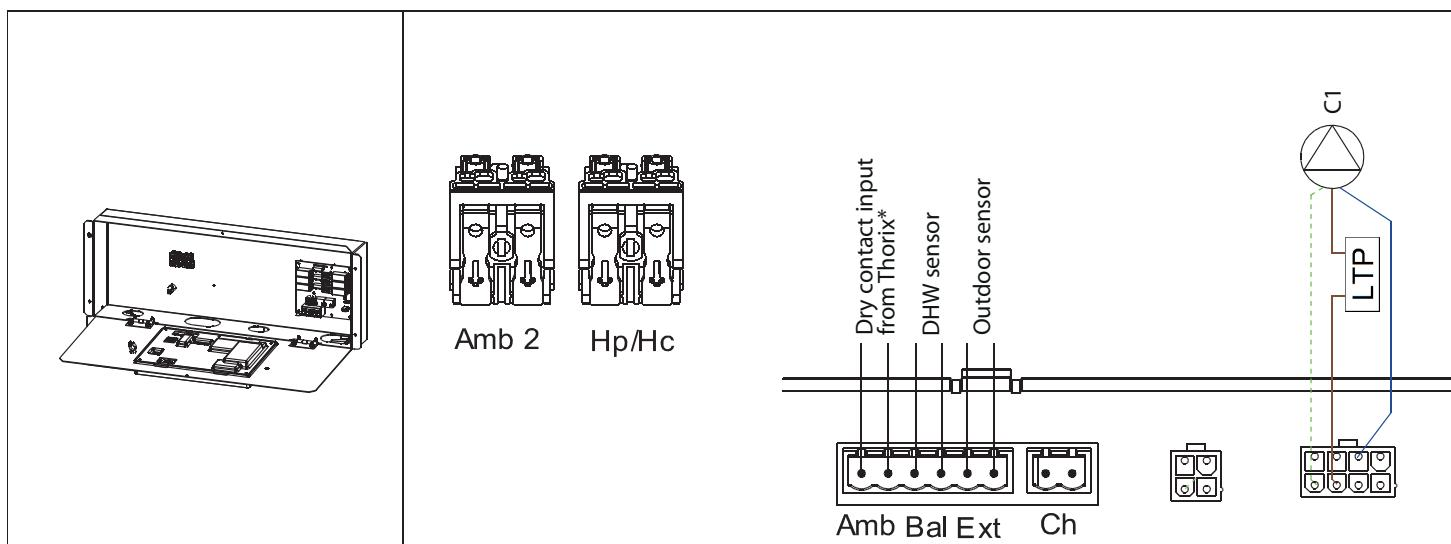
\* On the Thorix module, connect the two wires to the Alarm output and set P219=1.
