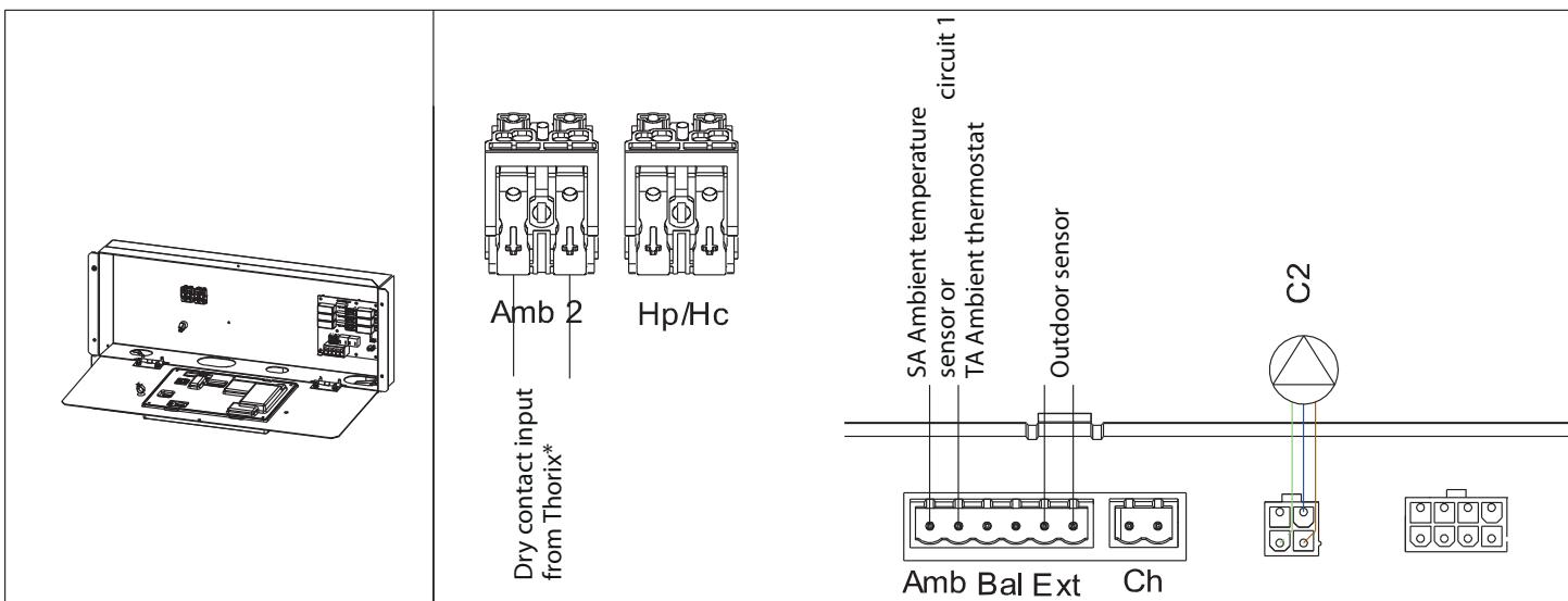
\* On the Thorix module, connect the two wires to the Alarm output and set P219=1.
