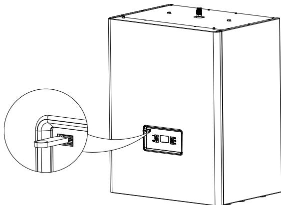
\* if the USB stick is not recognized, disconnect and reconnect the electrical supply to the appliance and try again.
