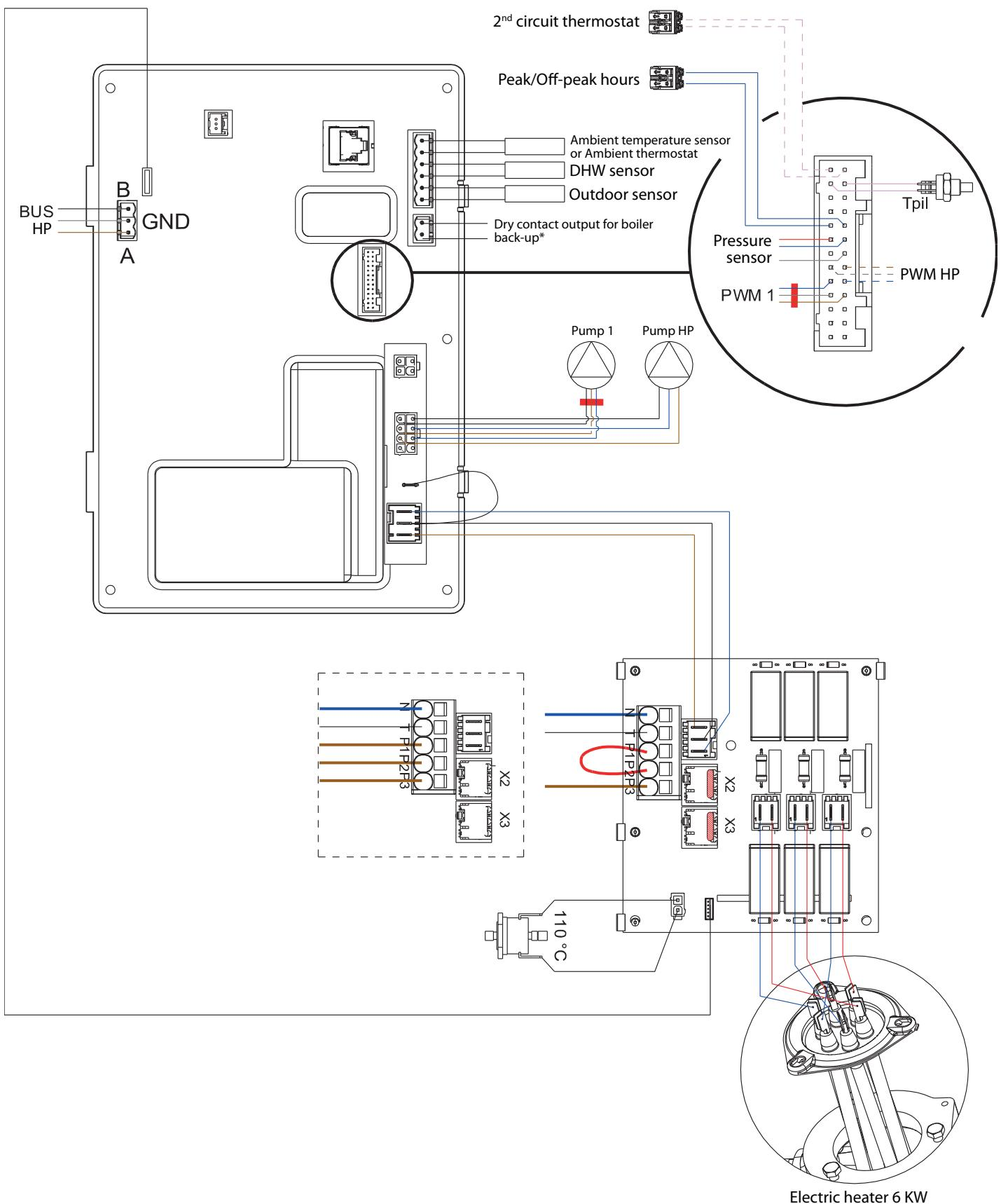
\* Dry contact to be connected to the ambient thermostat input of the boiler back-up.
