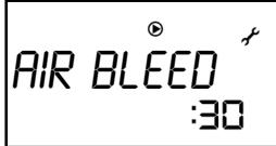
The purging cycle activates the circulator pump at an alternating rhythm to allow the displacement and purging of any air bubbles accumulated at high points of the installation using the **Pilot's** automatic purger.
