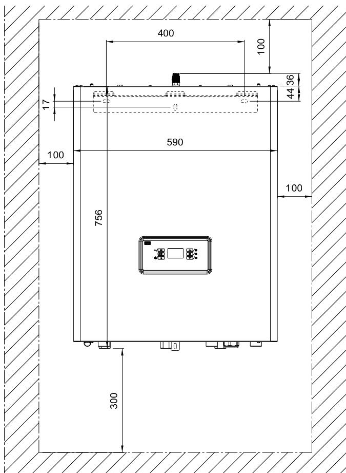
The wall bracket must be fixed to the wall.
